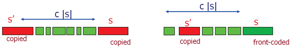
FIGURE 6.4: The two cases occurring in LPFC. Red rectangles are copied strings, green rectangles are front-coded strings.
