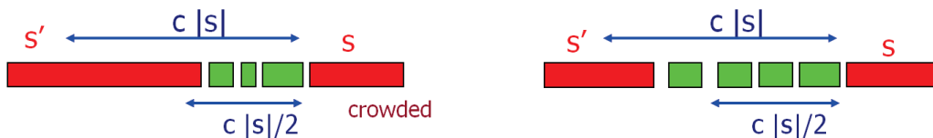
FIGURE 6.5: The two cases occurring in LPFC. The green rectangles denote the front-coded strings, and thus their FC-characters, the red rectangles denote the two consecutive copied strings.
