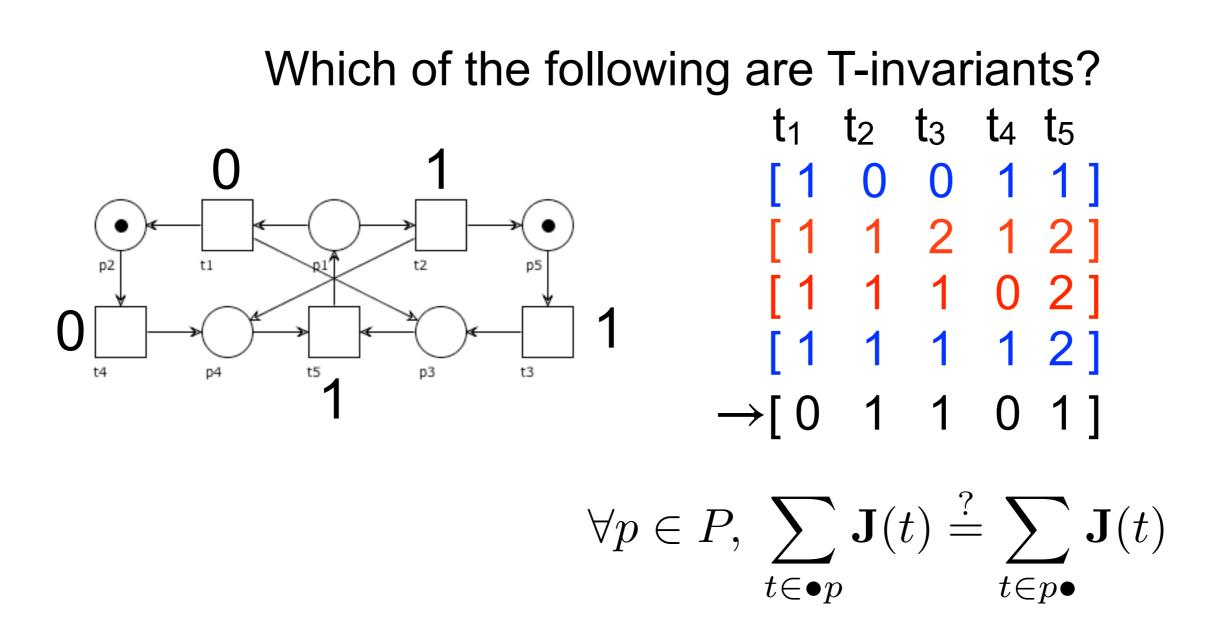
Which of the following are T-invariants? t<sub>1</sub> t<sub>2</sub> t<sub>3</sub> t<sub>4</sub> t<sub>5</sub> [1 0 0 1 1] [1 1 2 1 2] p2 t1 t2 p5 [1 1 1 0 2] [1 1 1 1 2] t5 р3 t3 t4 p4 1
