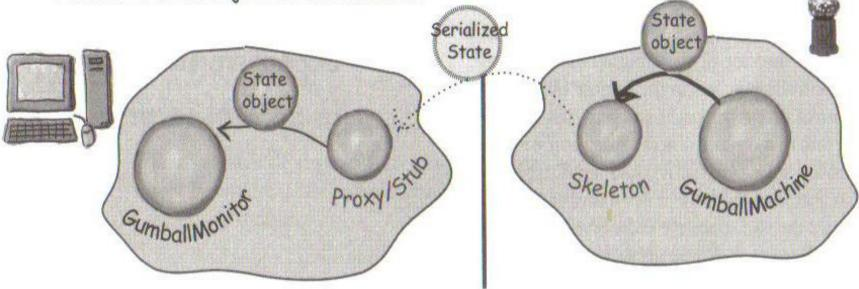
The monitor hasn't changed at all, except it knows it may encounter remote exceptions. It also uses the GumballMachineRemote interface rather than a concrete implementation. Likewise, the GumballMachine implements another interface and may throw a remote exception in its constructor, but other than that, the code hasn't changed.
