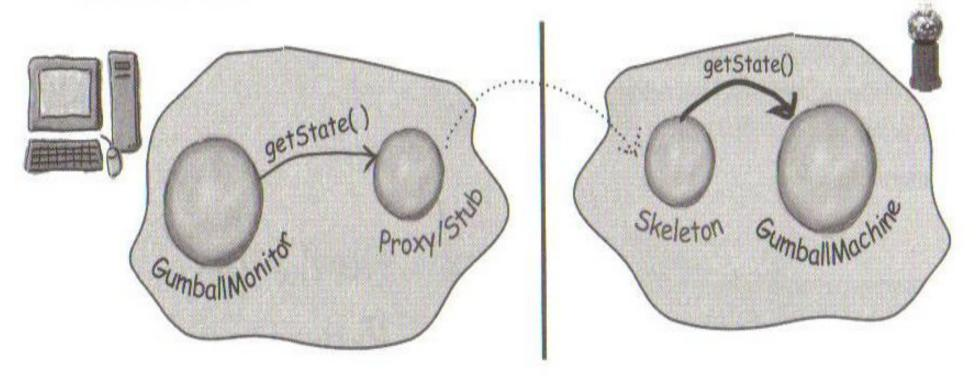
GumballMachine returns the state to the skeleton, which serializes it and transfers it back over the wire to the proxy. The proxy deserializes it and returns it as an object to the monitor.
